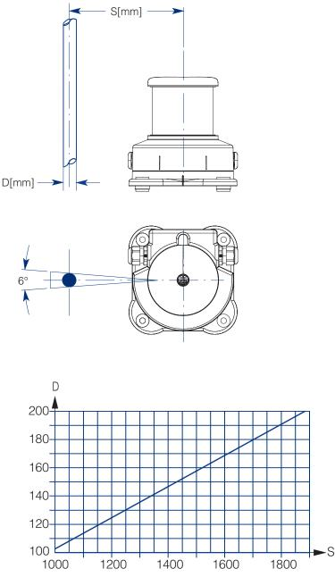
Diagram for choosing the minimum distance between obstacle and mounting plate.
